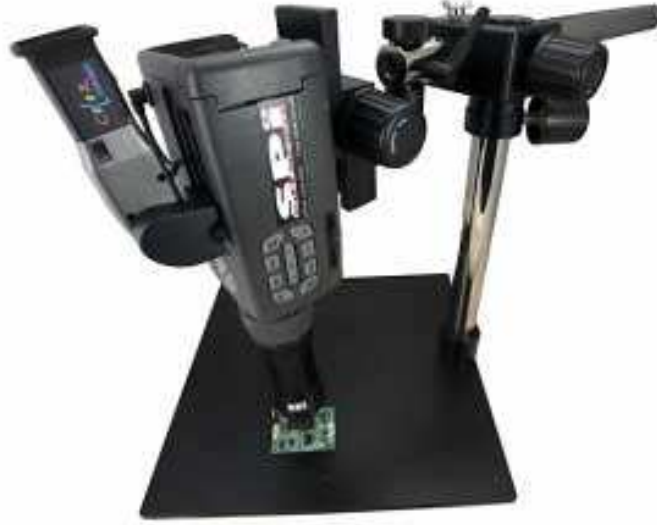
Figure 3.6 Infrared (IR) thermal microscopy setup.
